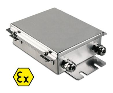
Stainless steel junction box with IP66 protection from water and dust, and fitted with an intrinsically safe electronic board for junction and equalisation of load cells. Terminal boards with screws for easing th connection of the load cells and signal adjustment trimmer, for an accurate and reliable equalisation. Marking: ATEX II 2G Ex ib IIC T6 Gb for gases.
